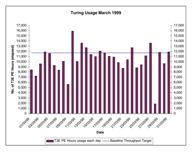
The above usage graph for the Turing system shows that the overall workload tailed off towards the end of each week. This resulted in the system running, on average, under baseline.
