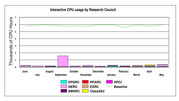
The above graph shows the historic interactive usage of the Origin 300 system (Wren). Eight of the higher speed 500Mhz CPUs in Wren deliver the baseline capacity equivalent to that which was previously available on the Origin 3000 system (Fermat) for interactive usage.
