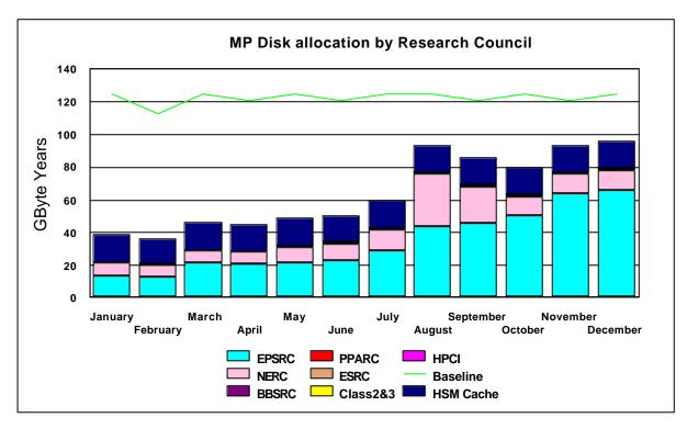
The graph above illustrates the historic allocation of the Medium Performance Disk on Fermat. From July 2000, 200 Gbytes has been used as a data cache for the enhanced HSM system.
