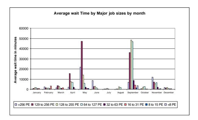
It can be seen from the above graph that the additional capacity added to the service, in the shape of the upgrade to Fermat and the addition of the Origin 3000 (Green), are now reducing the burden on the T3E (Turing) and reducing the queue wait times.
