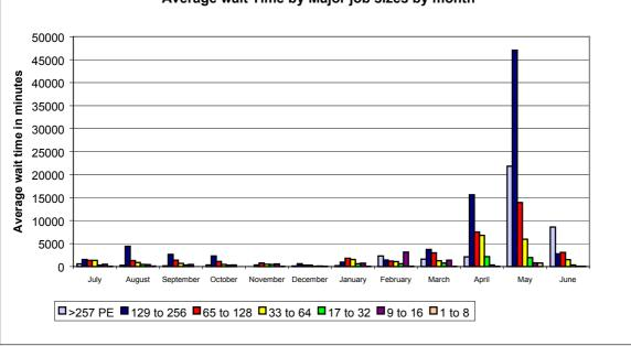
It can be seen from the above graph that the additional capacity added to the service, in the shape of the upgrade to Fermat and the addition of the Origin 3000 (Green), are now reducing the burden on the T3E (Turing) and reducing the queue wait times.
