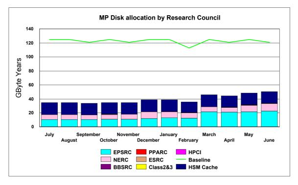
The graph above illustrates the historic allocation of the Medium Performance Disk on Fermat. From July 2000, 200 Gbytes has been used as a data cache for the enhanced HSM system.
