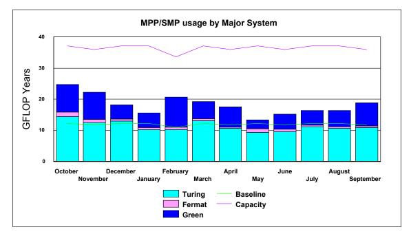
The next chart shows the historic interactive usage of the 'baseline' Fermat system (equivalent to 16@250Mhz CPUs) up to the end of February 2003, at which point the interactive usage was transferred to Wren and Fermat became a batch-only system. Eight of the higher speed 500Mhz CPUs in the Origin 300 system (Wren) deliver the baseline capacity equivalent to that which was previously available on Fermat for interactive usage.
