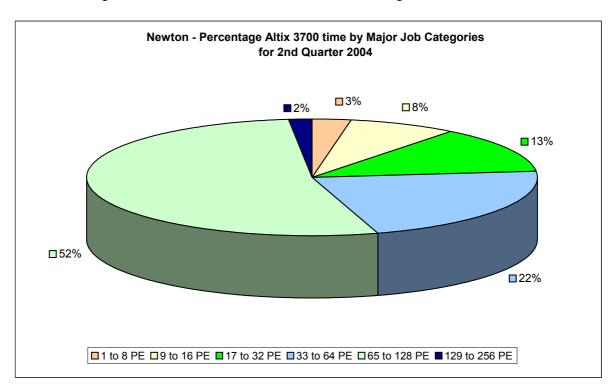
Newton's workload during the second quarter was focused largely in the 65 to 128 PE range, with significant volumes of application development work.
