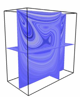
Figure 2. Flow profile for the central orthogonal slice for each of the three principal axes
