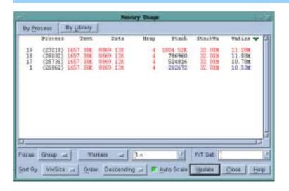
Clicking on a column heading sorts the information from maximum to minimum or vice versa. You can also sort information using the controls at the bottom of the window.
