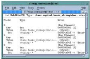
TotalView can transform STL vectors, lists, and maps using native and GCC compilers on IBM AIX, IRIX/MIPS, and HP Tru64 Alpha. It also supports GCC and Intel's Version 7 C++ 32-bit compiler running on Red Hat x86 platform.
