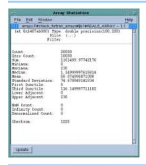
If you have added a filter or a slice, these statistics only describe the information currently being displayed; they do not describe the entire unfiltered array. For example, if 90% of an array's values are less than 0 and you filter the array to show only values greater than zero, the median value will be positive even though the array's real median value is less than zero.
