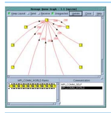
The numbers in the boxes indicate the MPI message tag number. Diving on a box tells TotalView to open a Process Window for that process.
