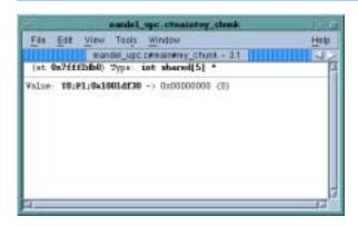
Because the Type field shows the full type name, TotalView is telling you that this is a pointer to a shared int with a block size of 5.
