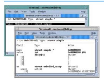
The nested dive window—displayed in the bottom right corner of the figure—shows the structure referenced by the simple\* pointer.
