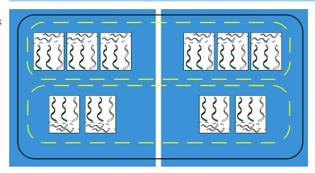
Figure 26 differs from Figure 25 in that it has ten processes executing within two processors rather than five processes within one processor. Although the number of processors has changed, the number of control and share groups is unchanged. This is not to say that the number of groups could not be different. It's just that they do not differ in this example.
