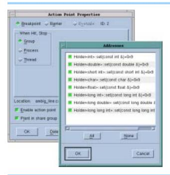
If TotalView cannot figure out which instantiation to set a breakpoint at, it will display its Address Dialog Box. (See Figure 131 on page 185.)
