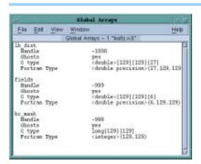
The arrays named in this window are displayed using their C and Fortran type names. Diving on the line containing the type definition tells TotalView to display Variable Windows containing information about that array. (See Figure 75.)
