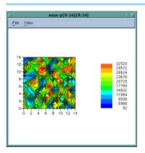
You can display random data by selecting only the **Zone** setting and turning **Mesh**, **Shade**, and **Contour** off. The display shows where the data is located, and you can click on the display to get the values of the data points.
