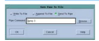
When piping information, TotalView sends what you've typed to /bin/sh. This means that you can enter a series of shell commands. For example, here is a command that ignores the top five lines of output, compares the current ASCII text to an existing file, and writes the differences to another file:
