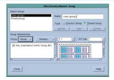
This dialog box can be divided into two halves. The top half allows you to add, update, and delete named sets. The bottom half contains controls that allow you to specify which processes and threads will become part of the group. These controls are discussed in the previous section.
