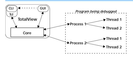
The CLI and the GUI are components that communicate with the TotalView core, which is what actually does the work. In this figure, the dotted arrow between the GUI and the CLI indicates that you can invoke the CLI from the GUI. The reverse isn't true: you can't invoke the GUI from the CLI.
