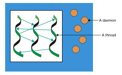
In this computing model, a program (the main thread) creates threads. If they need to, these newly created threads can also create threads. Each thread executes relatively independently from other threads. You can, of course, program them to share data and to synchronize how they execute.
