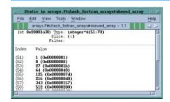
TotalView can visualize laminated variables. (See "Visualizing a Laminated Variable Window" on page 272.) The process or thread index will be one of the visualized data's dimensions. This means that you can only visualize scalar or vector information. If you don't want the process or thread index to be a dimension, use a nonlaminated display.
