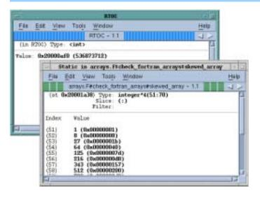
The top-left window shows the result of diving on a register, while the bottom-right window shows the results of diving on an array variable.
