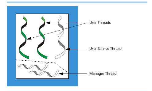
These service threads are, of course, also worker threads. They are called different things just to keep the different kinds of things that they do separate. As an example, this could be a thread whose sole function is to send data to a printer in response to a request from the other two threads.
