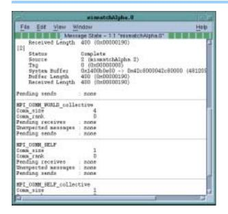
tor structures, TotalView displays both of them. One will be used for point-to-point operations and the other for collective operations.
