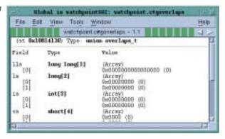
When TotalView displays some complex arrays and structures, it displays the compound object or array types in the Variable Window.
