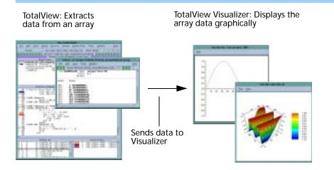
Configuring TotalView to Launch the Visualizer TotalView launches the Visualizer when you select the Tools > Visualize command from the Variable Window. It will also launch it if or when you use a \$visualize function within an evaluation point and the Tools > Evaluate Dialog Box.
