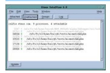
Normally, the first MPICH process is the highest process with the correct image name in the process list. Other instances of the same executable can be:
