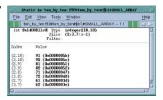
After you enter this slice value, TotalView only shows elements in rows 2 and 3 of the array, beginning with column 10 and ending with column 7.
