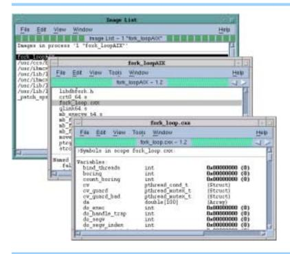
The screen in the upper-left corner shows a Variable Window created by diving on one of the files in Figure 153 on page 233. The center screen dives on a block in that subroutine. Finally, the screen in the lower-right corner shows a variable. (These screens were created using the View > Dive Anew command.) If you just dived on a line in a Variable Window, the new contents replace the old contents, and you can use the dive/undive icons to move back and forth.
