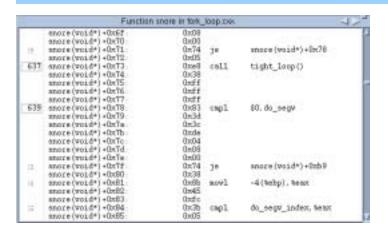
The final "assembler" figure (see Figure 126 on page 177) shows the split Source Pane, with one side showing the program's source code and the other showing the assembler version. In this example, the assembler is shown symbolically. How it is shown depends upon whether you've selected View > Assembler > By Address or View > Assembler > Symbolically.
