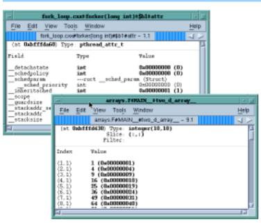
Because the data displayed in a Variable Window may not be simple, you can *also* dive on data in the Variable Window. When you dive in a Variable
