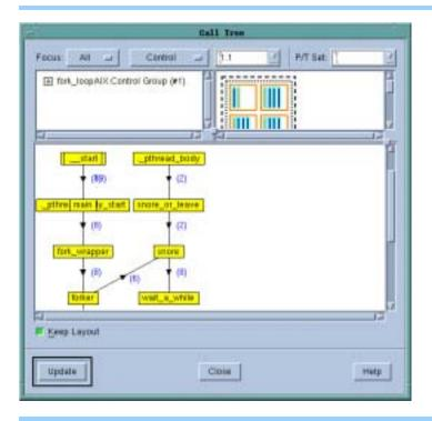
these controls, TotalView displays a call tree for the group defined in the icon bar of your Process Window. If TotalView is displaying the call tree for a multiprocess or multithreaded program, numbers next to the arrows indicate how many times a routine is on the call stack.
