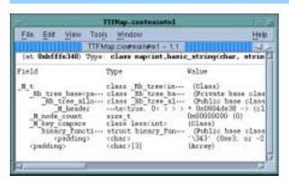
TotalView comes with a set of transforms that changes how it displays some STL data. For example, Figure 147 shows the transformed map.
