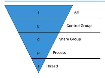
Notice that the " $\mathbf{g}$ " specifier indicates control and share groups. This inverted triangle is indicating that the arena focuses on a greater number of entities as you move from thread level at the bottom to "all" level at the top.
