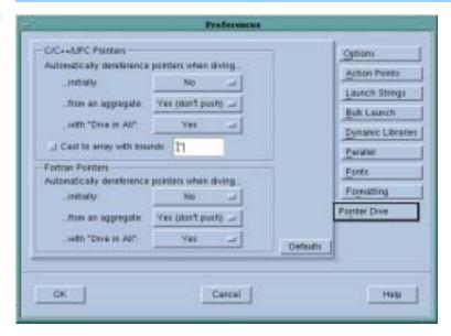
This preference is especially useful when you want to visualize data that is linked together with pointers, as it can present the data as a unified array. Because the data appears to be a unified array, you can use TotalView's array manipulation commands and the Visualizer to view this data.
