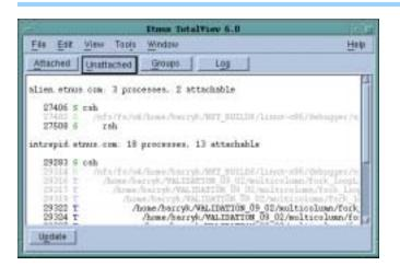
If you're debugging a remote process, the Unattached Page also shows processes running under your username on each remote host name. You can attach to any of these remote processes. For more information on remote debugging, refer to "Setting Up and Starting the TotalView Debugger Server" on page 61 and "TotalView Debugger Server (tvdsvr) Command Syntax" in the TotalView Reference Guide.
