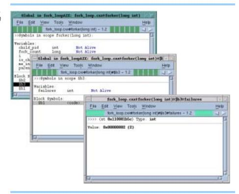
Window shows the name, address, data type, and value for the object. (See Figure 154.)
