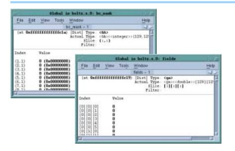
After TotalView displays this information, you can use other standard command and operations upon the array. For example, you can use the slice and filter operations and the commands that visualize, obtain statistics, and show the nodes from which the data was obtained.
