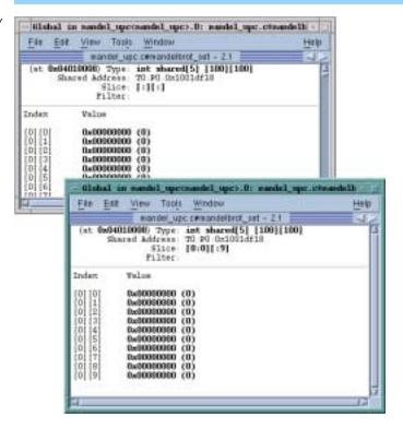
In this illustration, TotalView displays the value of a pointer-to-shared variable whose target is the array in the **Shared Address** area. As usual, the address within the process is shown in the top left of the display.
