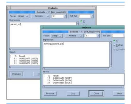
See Chapter 11, "Using Groups, Processes, and Threads," on page 197 for information on using the P/T set controls at the top of this window.
